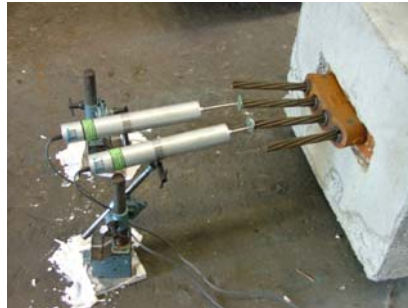
Setting the dial gauges to measure elongation of the wire strand
