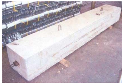
Test of load efficiency and of elongation of the anchored tendon
